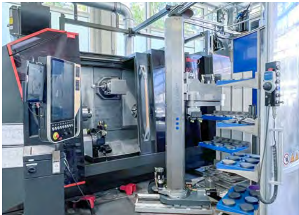
With workpiece pool for unmanned production
