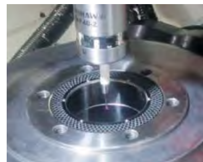
Determination of change in inner diameter by means of measuring probe
