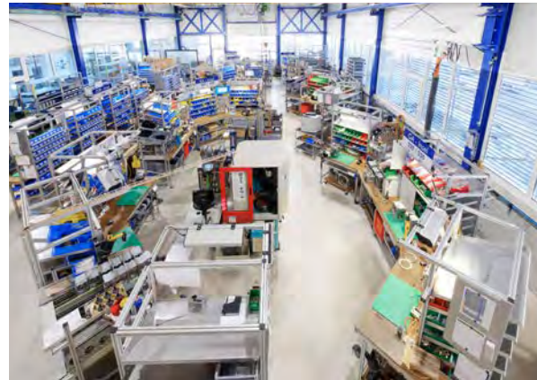
Assembly area with Kanban System
